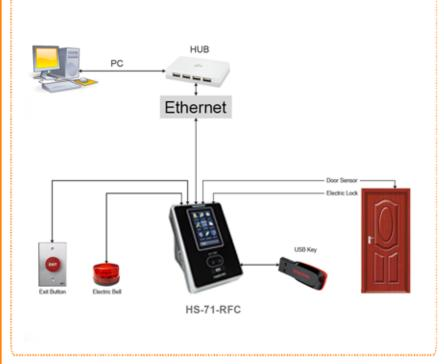
HS-71-RFC is a latest technological advancement using Facial Recognition suitable for both Time Attendance and Access Control and it is IP based device and that our Cloud based software can handle records from multi location
